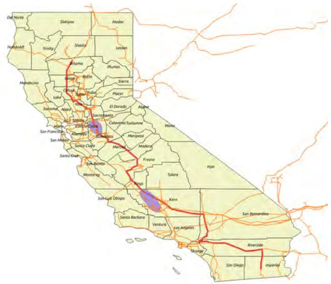
**Figure 60.** Map of potential CO<sub>2</sub> trunk pipeline. California counties are shown with existing major natural gas pipelines in orange. Approximate proposed CO<sub>2</sub> storage areas are marked with purple ovals. The base case CO<sub>2</sub> pipeline is shown in red. This route follows major natural gas pipelines and passes through our studied storage sites in the central valley, and a potential geothermal-powered direct air capture plant near the Salton Sea.
