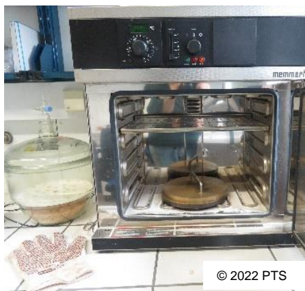
Figure 25: Drying oven used for the sheet adhesion test.
