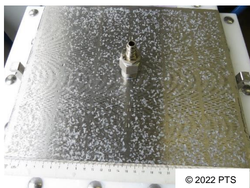
Figure 38: Macro stickies screening reject on the 150 \mu\text{m} plate.
