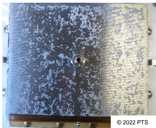
Figure 32: Fine reject on the 150 µm plate.
