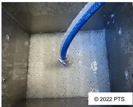
Figure 17: Coarse reject after the water draining.
