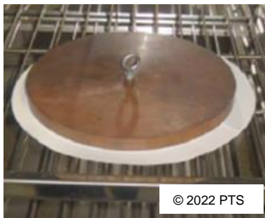
Figure 26: Lab sheet with carrier board and cover sheet placed between metal plates into the oven.
