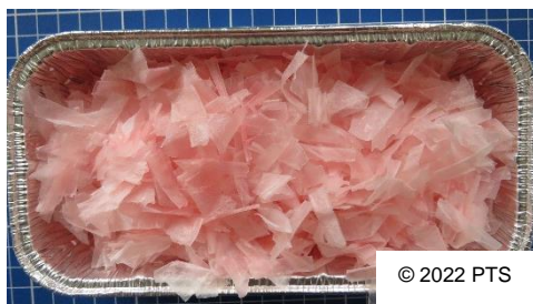
Figure 22: Coarse reject dried in the aluminium tray.
