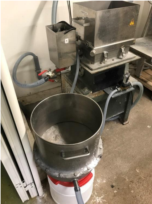
Figure 2.C. Top view of thickener as used in CTP
