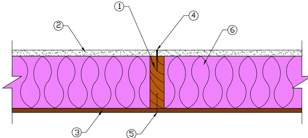
1. **Framing:** Nominal 2x6 wood studs, spaced 24 in. o.c., double top plates, single bottom plate
