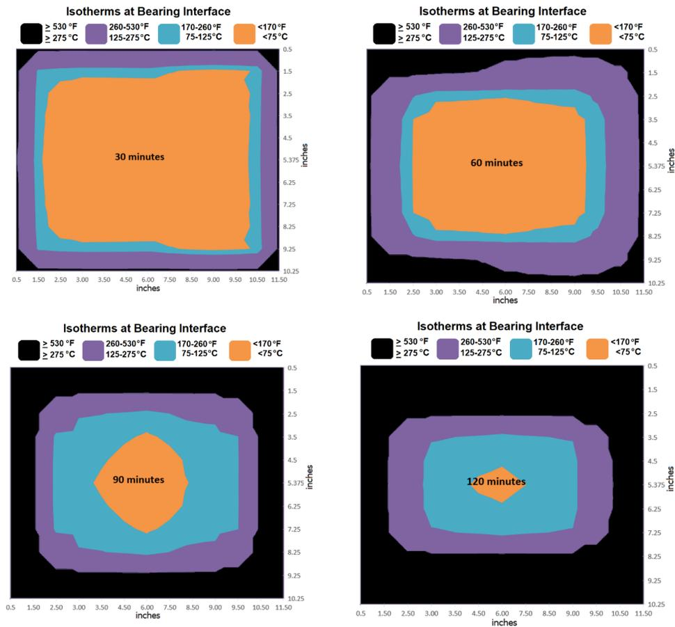
Based on this thermocouple data, a regression was developed to predict the depth of the  $212^\circ\text{F}$  isotherm relative to  $a_{\text{char}}$ . The depth of the  $212^\circ\text{F}$  isotherm was estimated to be at a depth of  $1.6a_{\text{char}}$  ahead of the char front.
