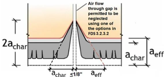
When gaps between mechanically-laminated decking are unobstructed, such as can occur when the decking is untopped, hot gases will pass through the gaps, and the sides of the decking members will char. This charring can be approximated assuming the sides of a member, char to a depth of  $a_{eff}$  with dimension as shown in Figure C3-8.
