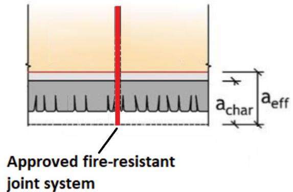
C3.2.3.2 Intersections and abutting edges of exposed members that are in contact or have gaps less than or equal to 1/8 inch and where air flow through gaps is permitted to be neglected using one of the options in FDS 3.2.3.2 (see Figure C3-3):
