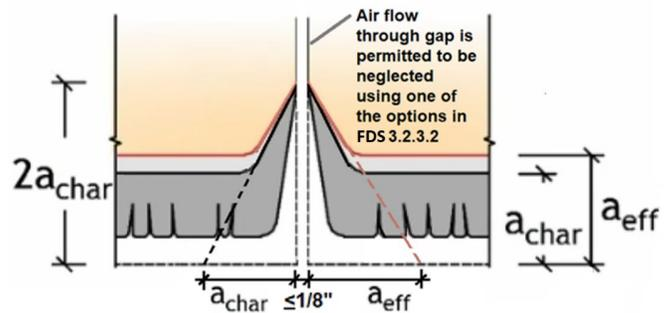
C3.2.3.3 Intersections and abutting edges of exposed members that are in contact or have gaps less than or equal to 1/8 inch but air flow through gaps is not permitted to be neglected (see Figure C3-4):
