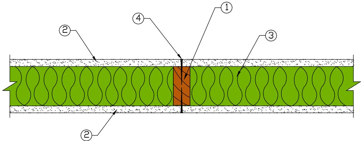
1. **Framing:** Nominal 2x4 wood studs, spaced 16 in. o.c., double top plates, single bottom plate
