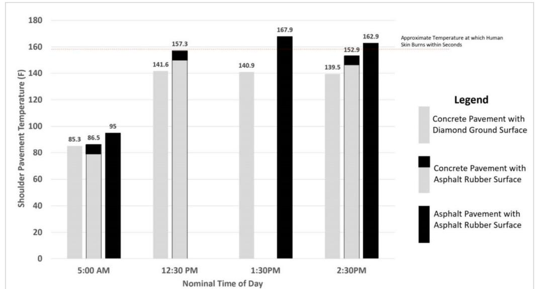
» Pavement shoulder temperatures for three pavement structures from a drone infrared test. The roadway's shoulder best represents the heat disparity among surface types because it is a non-trafficked area with minimal convection cooling from traffic.
