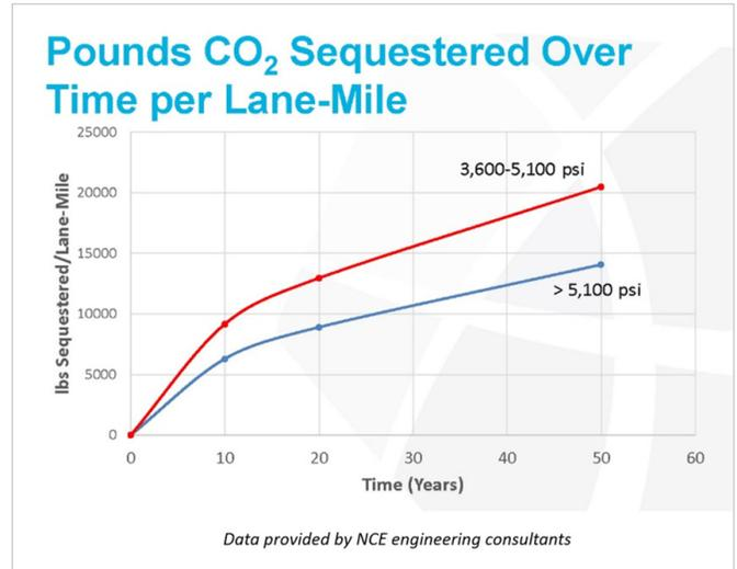
» Over a time span of 50 years, concrete achieves carbonation of roughly 14,000 to 20,000 pounds per lane mile.
