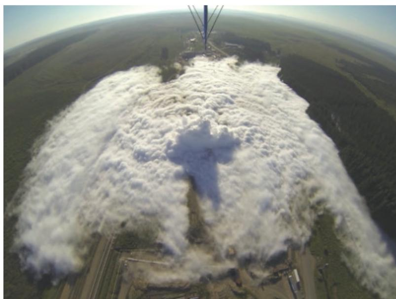
CO<sub>2</sub> cloud from a rupture test performed at DNV GL Spadeadam, Photo: DNV GL
