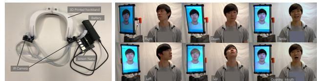
**Figure 5: The NeckFace system. We show the shoulder pad used to hold the cameras and the illumination sources as well as the computing module (Left). Several examples of facial poses and expressions and how they are rendered on our articulated display (Right).**
