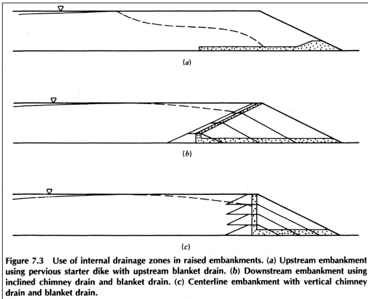
**Figure A6.** It is possible to install blanket drains using all three construction methods, although chimney drains can be installed using only the downstream and centerline construction methods. These drains lower the water table and reduce the likelihood of internal erosion of the tailings dam, seismic or static liquefaction of the tailings dam or tailings deposit, and failure of the foundation under the tailings. Figure from Vick (1990).
