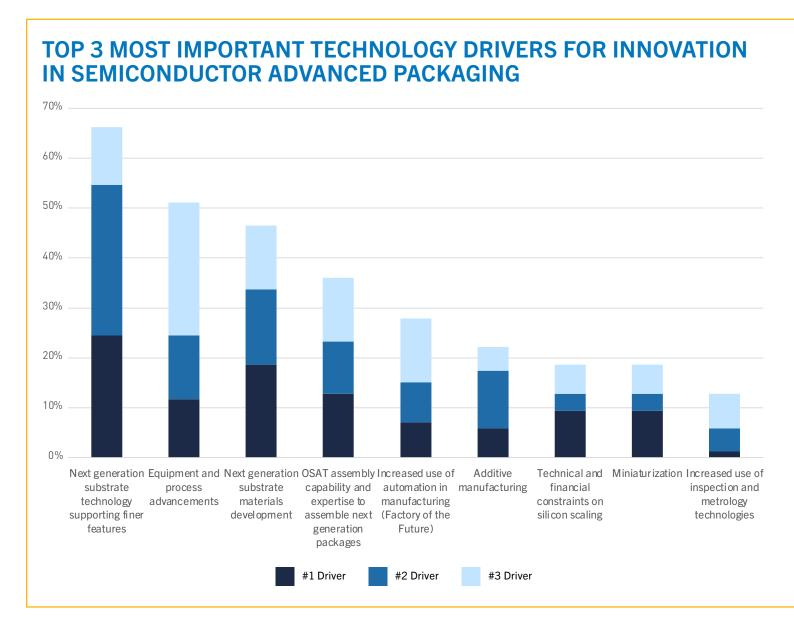
Next-gen substrates will be needed for the next-gen products. Being able to implement finer features on an IC substrate carries many benefits. It can dramatically reduce the size, weight, and packaging needed, which in turn increases the electronic content within an existing space. Moreover, supporting finer features allows for a reduction in the number of microvia layers required, which reduces cost and improves reliability.
