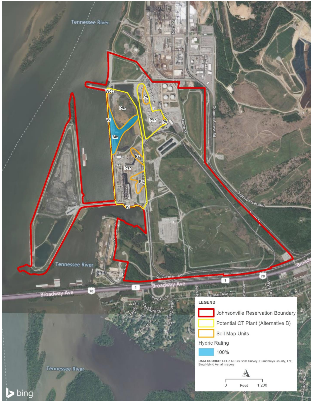
Figure 3.5-8. Soils on the proposed CT plant site on the Johnsonville Reservation
