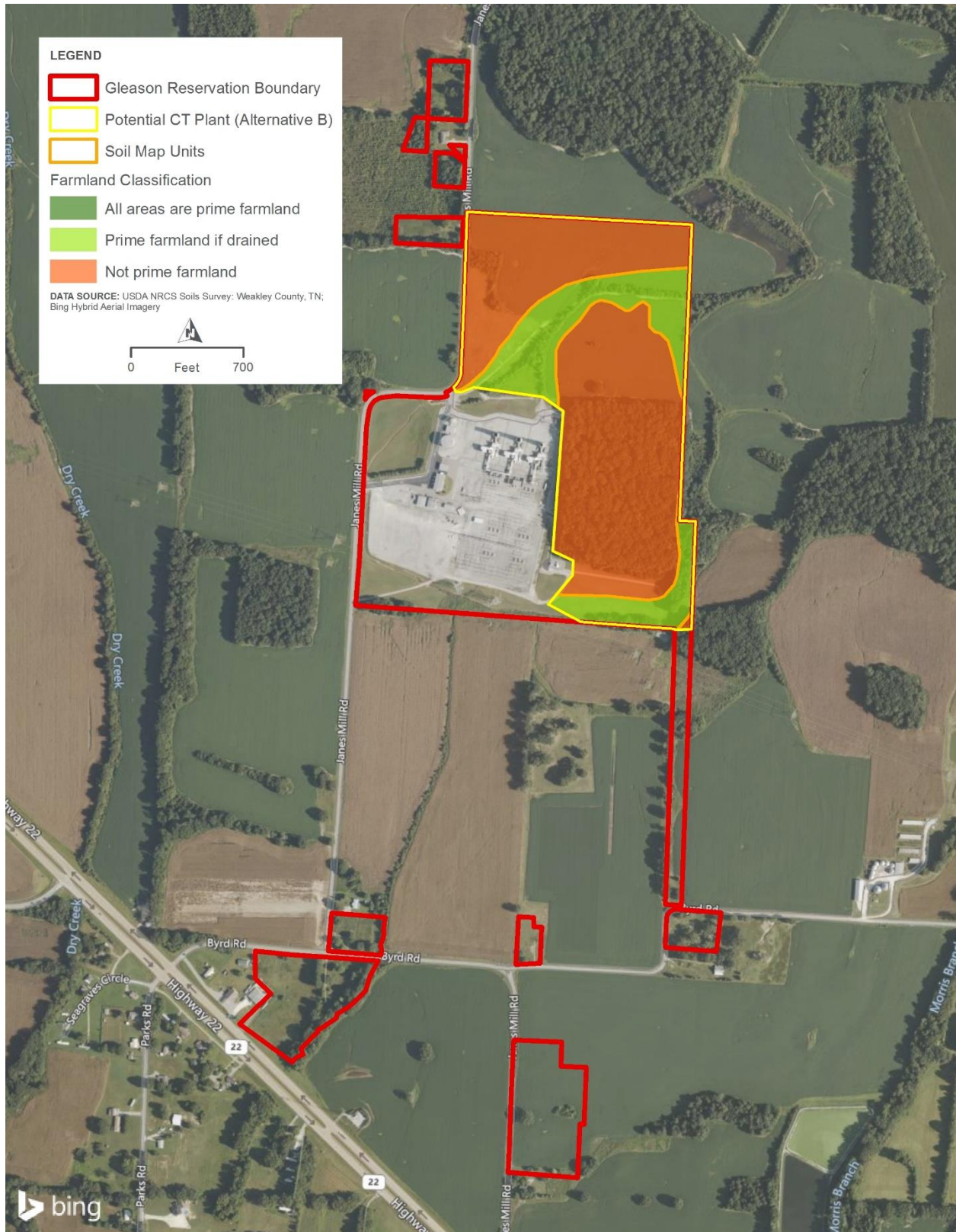
Figure 3.5-11. Soils classified as prime farmland on the proposed CT plant site on the Gleason Reservation
