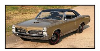
In late 1963, John DeLorean and his engineering team developed the GTO as a performance option for the lightweight Pontiac Tempest. Powered by a tuned 389 cubic inch V-8 engine, the original GTO combined great acceleration, aggressive handling, and handsome styling.
