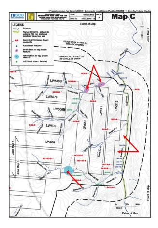
Figure 1: A section of the proposed mine layout for Area 5 showing the three different types of setbacks on which the mine plan is based.
