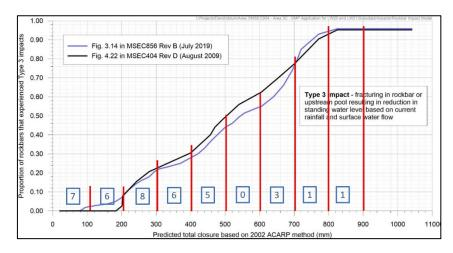
Figure 5: Ranges in predictions of valley closure for key stream pools on drainage lines plotted on MSEC rock bar model.
